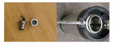
Install the o-rigs on the plugs (posts) if not already installed and place the small poppet valves in the liquid and gas plugs (posts).
