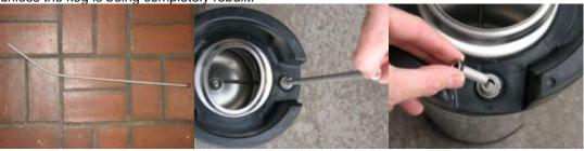
Slide the o-ring on the long liquid dip tube and insert the dip tube into the keg through the 'out' port. The end of the tube will usually angle in to the centre of the bottom of the keg. Slide the o-ring on the short gas dip tube and insert the tube into the 'in' port.
